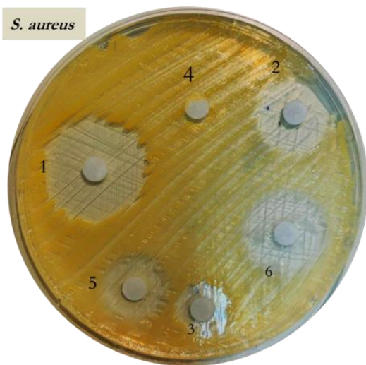
Figure 2: Inhibition growth zone test of disinfectants and antiseptics used in the study toward S. aureus . H 2 O 2 3% [1], 10% Orolin [2], 100% CHX [3], 84 Disinfectant 1% [4], 100% Actosal [5] and 70% Ethyl alcohol [6].
